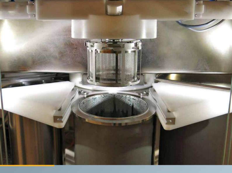
The UCMIndexLine is a very compact rotary indexing system with six cleaning stations for precision cleaning on an aqueous basis. With the integrated cleaning and rinsing stations, with and without ultrasound, almost all processes can be mapped. Thus, any process sequence as well as any number of process sequences can be represented. The system is especially designed for very small and complex components.
