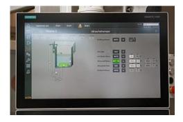
During analysis and evaluation by the software, the measured values are compared with the target parameters defined as reference values for the respective treatment station, in this case the bottom-mounted ultrasonic transducer.
