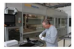
Ultrasonic power and frequency have a decisive impact on the cleaning effect. These process parameters are therefore checked for correct functioning once a year as part of a service agreement with a portable version of the APM system.
