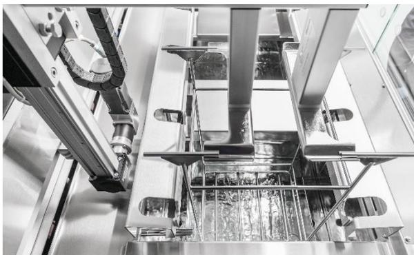
The standard automatic transport system has a servo drive for exceptionally gentle workpiece transport and part-specific lift-out for pre-drying parts as they leave the last tank.
