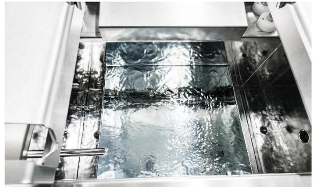
All wet-stage tanks of the system, which is entirely made from electro-polished stainless steel, have a two-sided overflow which ensures the immediate removal of detached particles and other contaminants. This minimizes the risk of recontamination when the parts are moved.
