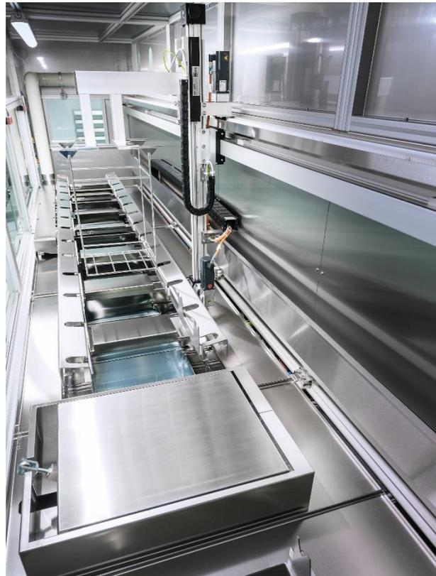
Up to nine cleaning and rinsing steps can be integrated into the cleaning system and variably equipped for use with mono, dual and multi-frequency ultrasonics.
