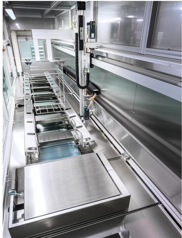
Up to nine cleaning and rinsing steps can be integrated into the cleaning system and variably equipped for use with mono, dual and multi-frequency ultrasonics.
